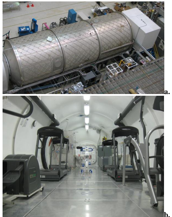
Figure 3. Regenerative ECLSS Module Simulator chamber. a) exterior view, b) interior view.
